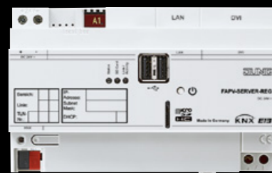
The Compact DIN C-rail PC Facility Pilot Server.
